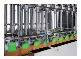
The linear filler has eight filling positions and is equipped with 1 l-metering cylinders.
