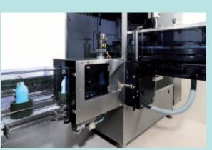
The empty containers that are supplied in bulk reach the pre-sorter of the Bottlemat via an elevator (left).
