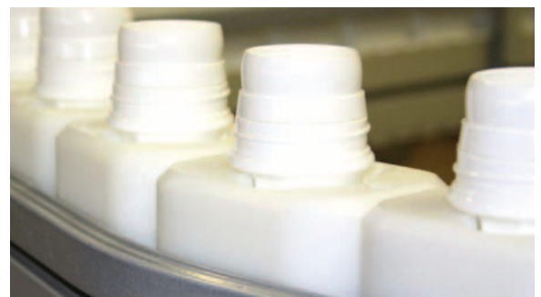
Since every container is guided individually, the Ratilight puck system is particularly suitable for the filling and closing of asymmetrical bottles.
